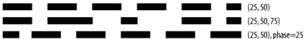
Figure 4-6. Line dash patterns: each line is 400 points long with a line thickness of 10 points
