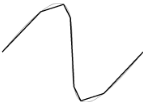
Figure 4-5. The thinner, smooth curve has a default flatness of 0.6; the thicker curve has a flatness of 100
